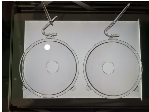
Fig. 7 Fresnel lens using polariscope to determine the optical characteristic
