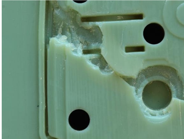
Figure 8: Avulsion failure region on the PRT insert from case study-2. This failure mode is characterized by progressive peeling of the substrate material. The image shows the catastrophic end state of the process.
