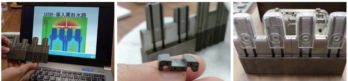
Fig. 4 Conformal cooling channel mold
