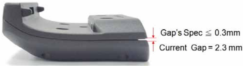
Fig. 1 The deformed situation of a real product showed 2.3mm which was over the spec. requirement.
