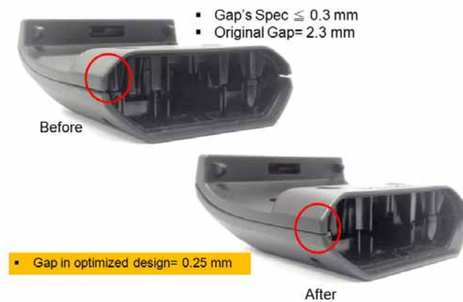
Fig. 11 The photo of actual molded part in original and optimized gap
