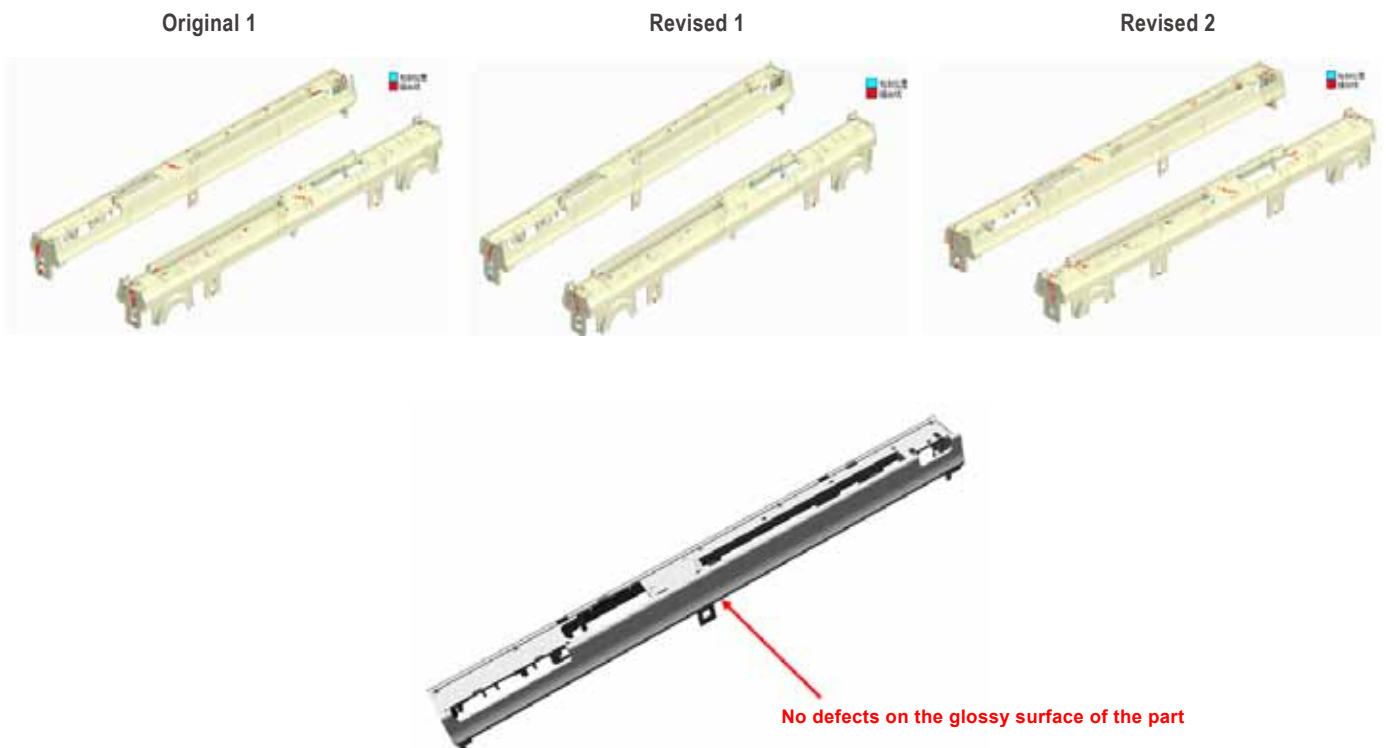
Fig. 7: No weld lines or air traps on the glossy surface of the part
