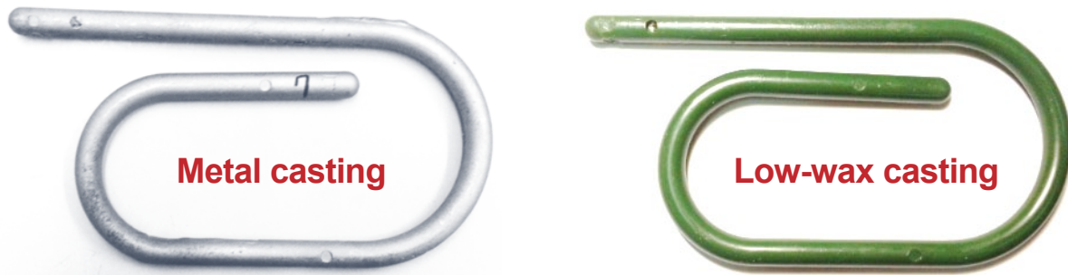
Fig. 7: Implementing GAIM technology in the wax injection can greatly improve the volumetric shrinkage by 48.7%.
