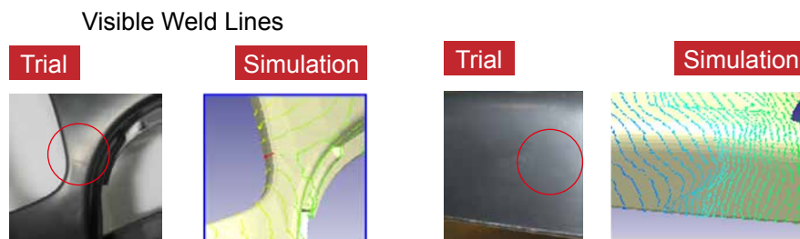
Figure 8: The weld line occurred in the actual injection trial (left) and some changes in gloss on the surface in the flow hesitation area were observed (right).
