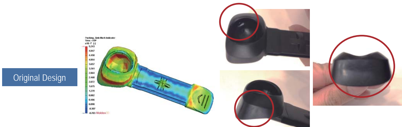
Figure 9: Moldex3D simulation analysis accurately predicted molding defects would occur in the socket region in the original design (left) and it was validated by the actual mold-trial result (right).
