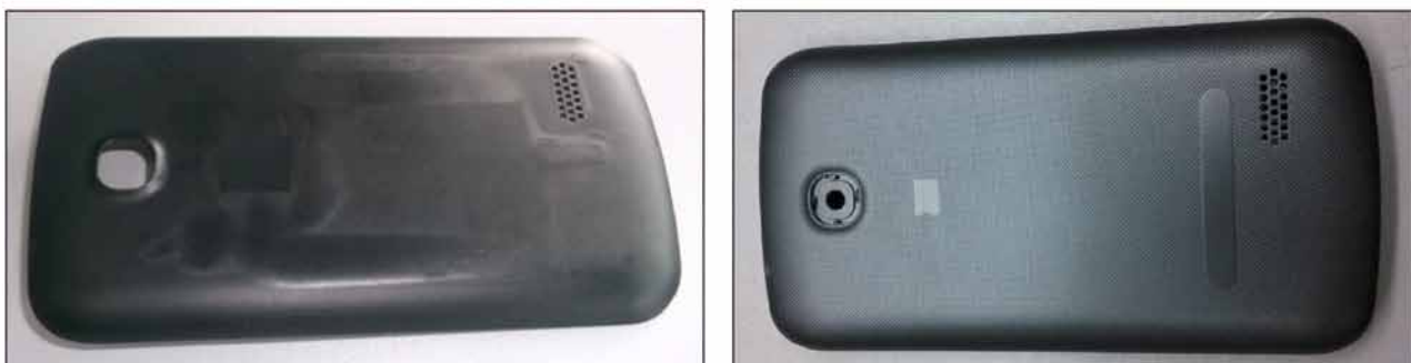
Fig 6. The actual mold trial results showed the original design has visible stress marks due to uneven thickness (left), and the optimized design does not have this issue (right). The actual mold trial results were strongly correlated with the simulation results.
