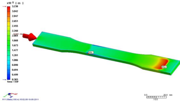
Fig. 9 Cell radius distribution of sample surface for 0.57 wt% N 2 SCF dissolved in PP. (Legend scale is 3.03 ~ 32.38 μ m)
