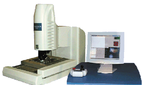
Figure 6. Micro-Vu with non-contact feature for warpage measurement.
