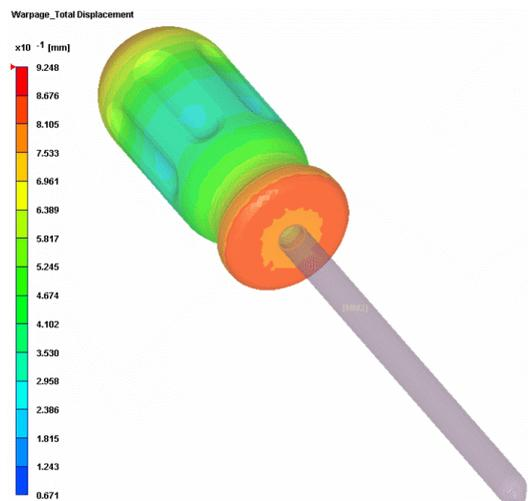
Figure 14. Total deformation of warpage analysis
