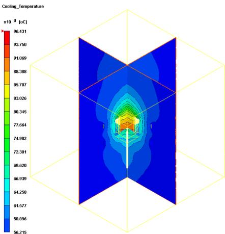
Figure 6-2. Temperature of moldbase at EOC (Insert Part: Beryllium\_Copper)
