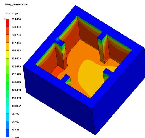
**Figure 4-3.** Temperature of cavity at EOF (Insert Part: Polymer)
