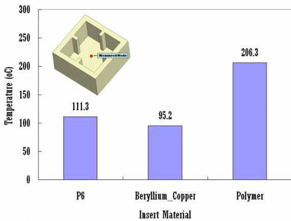
Figure 5. Comparison of temperature at EOF between different insert materials
