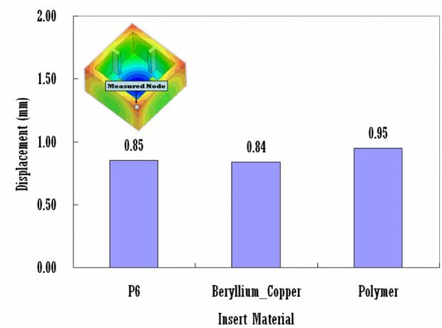
Figure 8. Comparison of warpage between different insert materials
