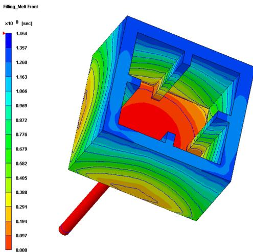
**Figure 3.** Melt front of filling analysis (Box)
