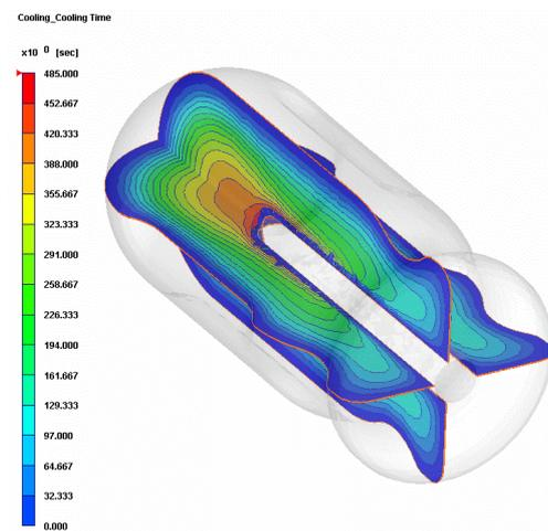
Figure 13. Predicted cooling time at EOC
