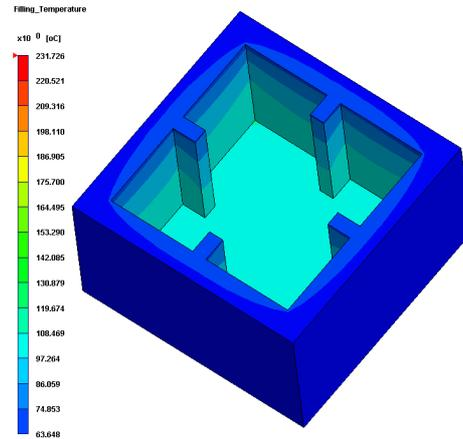
**Figure 4-1.** Temperature of cavity at EOF (Insert Part: P6)
