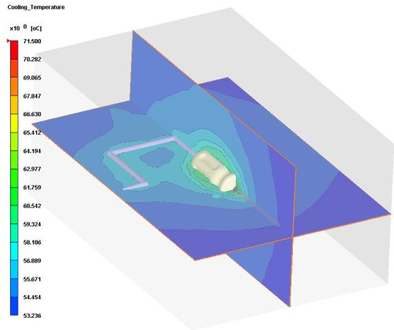
Figure 12. Temperature of moldbase at EOC
