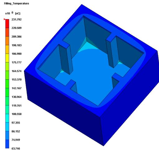
**Figure 4-2.** Temperature of cavity at EOF (Insert Part: Beryllium\_Copper)
