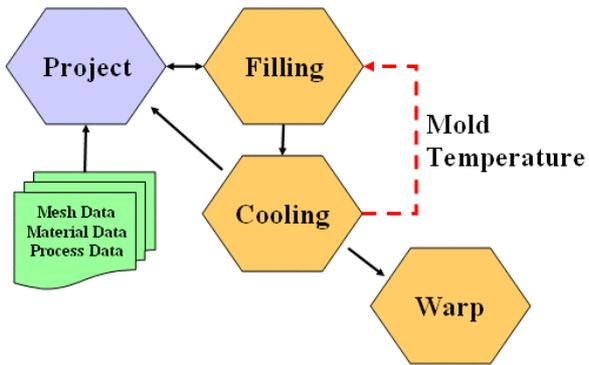
**Figure 1.** Computational framework of 3D injection molding analysis proposed in this work
