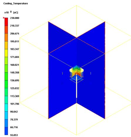
Figure 6-3. Temperature of moldbase at EOC (Insert Part: Polymer)
