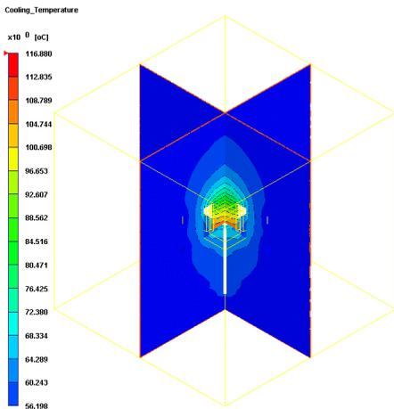
Figure 6-1. Temperature of moldbase at EOC (Insert Part: P6)
