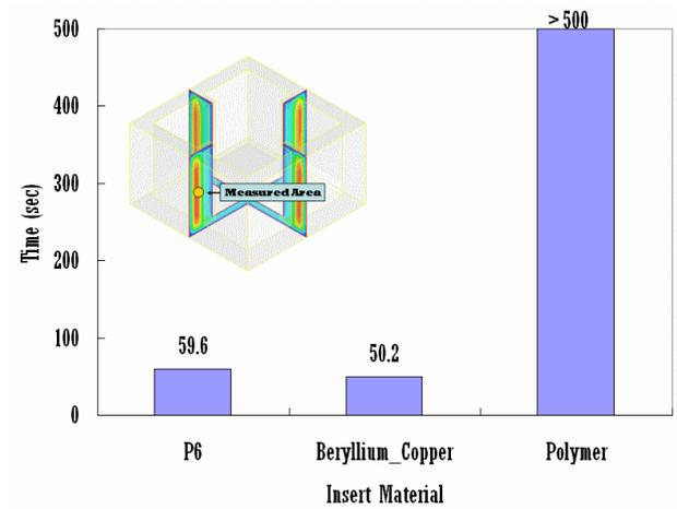
Figure 7. Comparison of predicted cooling time between different insert materials
