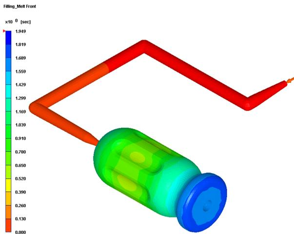
Figure 10. Melt front of filling analysis (Screw driver)
