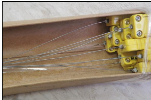
Fig. 6 Temperature sensor lines in the hot runner system
