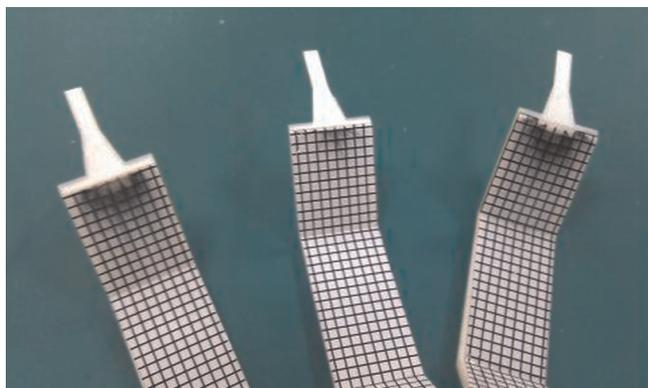
Fig. 6. Photographs showing the IMD injection molded parts
