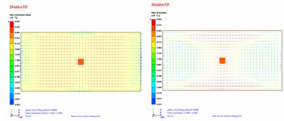
(a) On the wall (b) In the center cut plane
