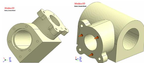
**Figure 5.** Throttle valve model with 3 gates
