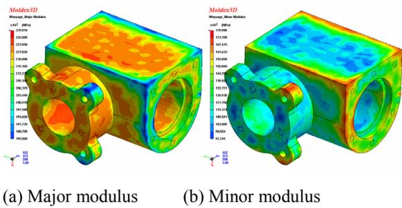
Figure 8. Predicted anisotropy mechanical modulus
