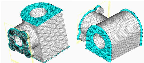
Figure 9. Constraint set for thermal stress analysis
