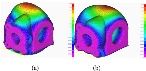
Figure 10. Deformation (a) simulation with fiber orientation effects (b) simulation with random orientation effects
