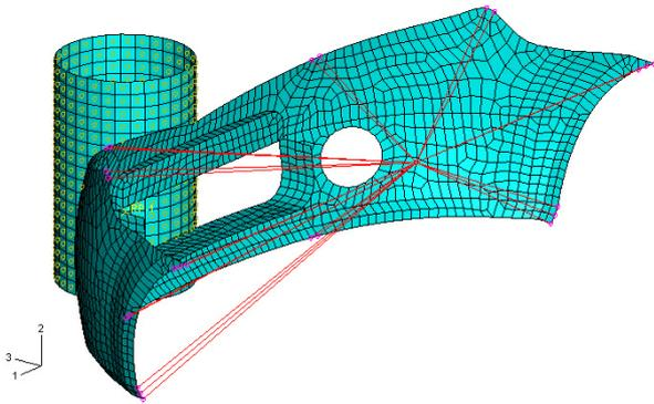
Figure 15. Models and constraints for impact analysis
