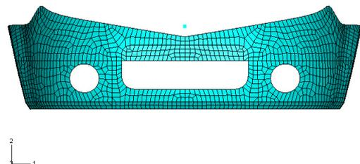
Figure 14. Specified mesh for impact analysis
