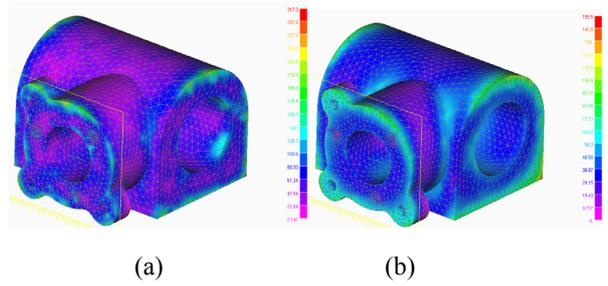
Figure 11. Von-mises stress (a) simulation with fiber orientation effects (b) simulation with random orientation effects
