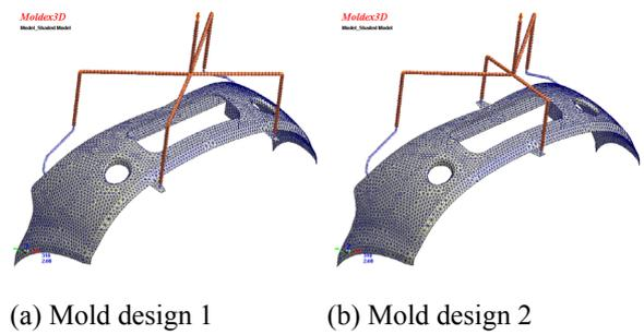
Figure 12. Bumper models with two mold designs
