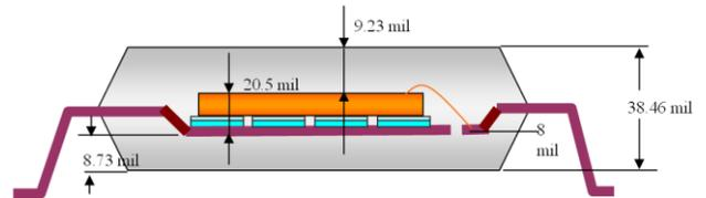
Figure 5. Side view of model geometry for paddle shift analysis
