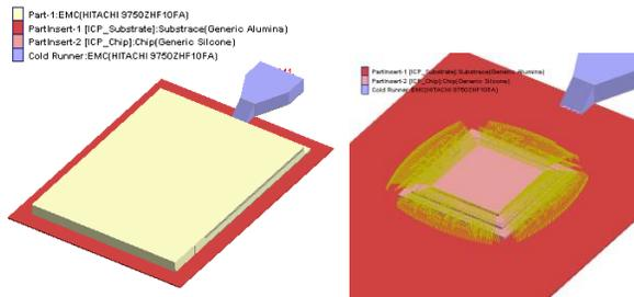
Figure 1. Geometry and wire layout of test model for wire sweep analysis
