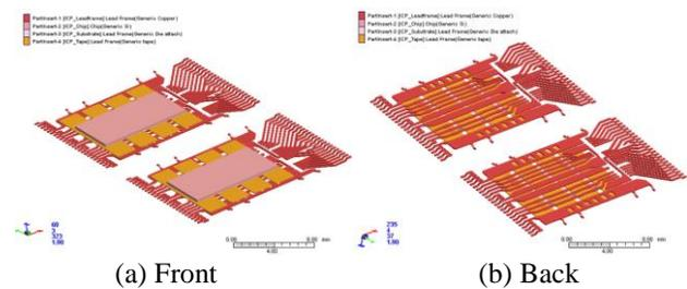
Figure 6. Top view of test model for paddle shift analysis
