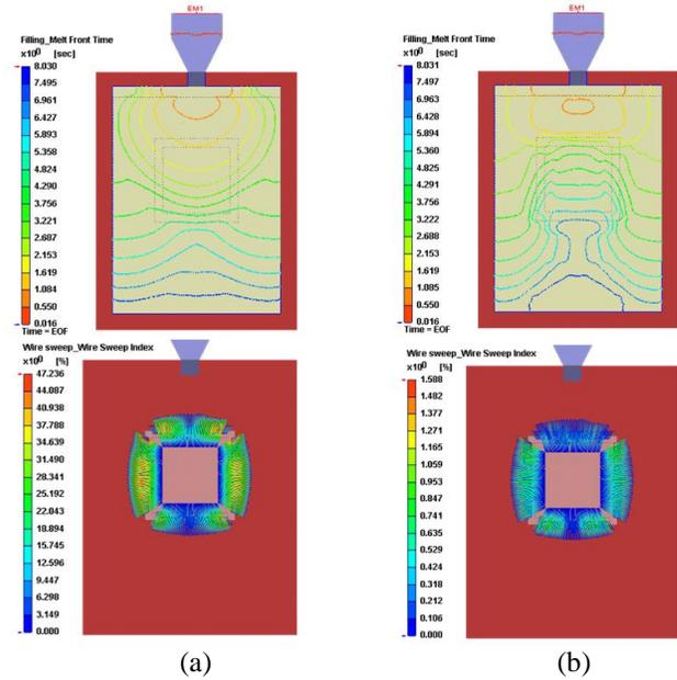
Figure 2. Contour of filling pattern and wire sweep index by (a) ignoring and (b) considering wire density effect
