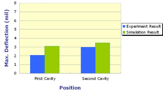
Figure 10. Comparison of maximum deflection of paddle shift between simulation and experiment results.
