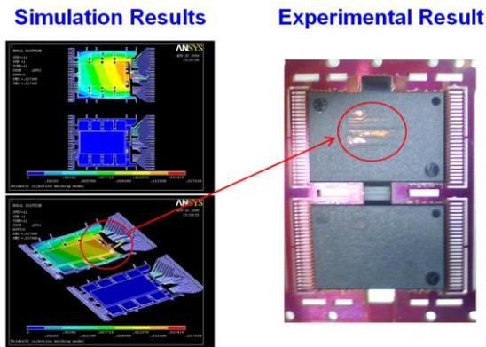
Figure 8. Comparison of deformed shape at end of filling between simulation and experiment results
