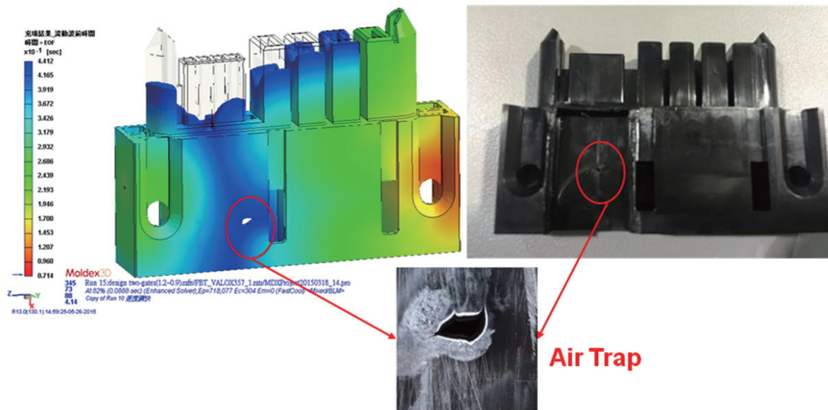
Fig. 7 Air trap comparison between the experiment and simulation results in Design 2
