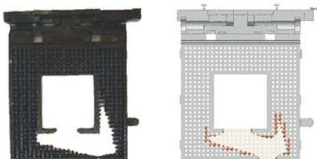
Moldex3D provides accurate simulations of flow patterns for plastic parts even with complicated geometry.
