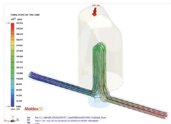
Figure2. Stream lines inside a baffle cooling channel
