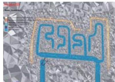
Fig. 1. Cooling channels and mold base – true 3D mesh model for simulation accuracy
