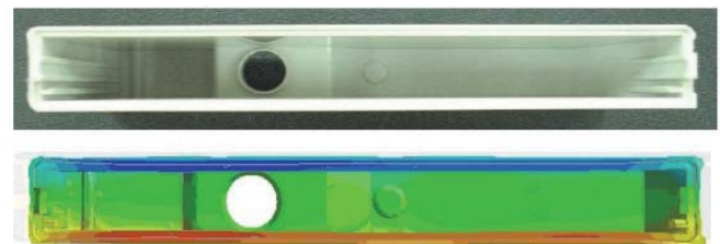
Fig. 5. Warpage results of revised design with conformal cooling –real injected part and simulation result
