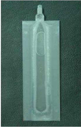
Figure 6. The molded part after the water assisted injection molding.
