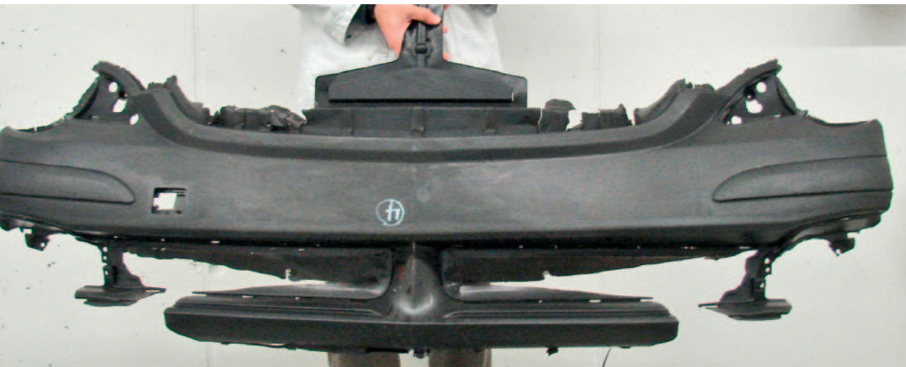
The 75 % filling of an injection molded front spoiler corresponds well with the result of a simulation (see bottom) (figures: SimpaTec, BASF Polyurethanes)
