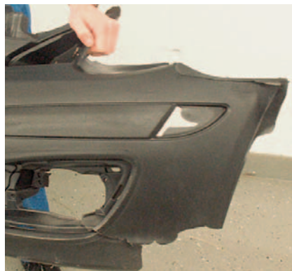
Fig. 2. Partially filled front spoiler obtained by "injecting into cross-linking material" after 1.4 s filling time
